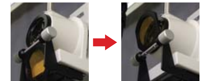
Yellow filter attachment (optional barrier filter) Fluorescence microscopy is possible with the built-in blue (exciter) filter.
